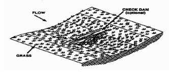
Figure: Swale Schematic
